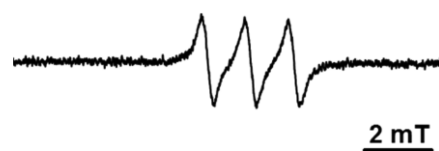
Figure 3. ESR spectra of a solution containing NOBL-1 (100 μM), FeSO 4 (1.5 mM), and N -methylglucamine dithiocarbamate (6 mM) in PBS (10 mM, pH 7.0, containing 1% DMF) after photoirradiation with blue light (470–500 nm, 200 mW/cm 2 ).
